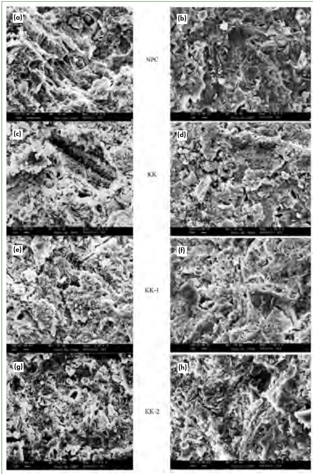
Fig. 3 Effect of TAK on cement paste microstructure at ((a), (c), (e) and (g)) 7 d and at ((b), (d), (f) and (h)) 28.
